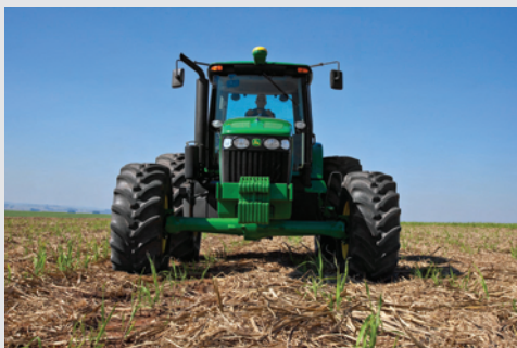
Tractor with front axle tread width up to 3 m.
