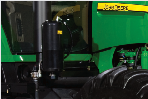
Pneumatic trailer air brake is factory installed.
