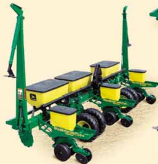
3 row 2,3m Planter with Vacuum seed metering and Dry fertilizer.
