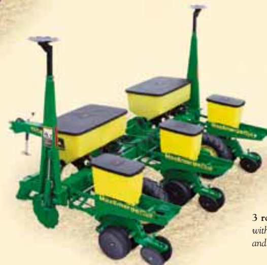
3 row 2,3m Planter with Vacuum seed metering and Dry fertilizer.
